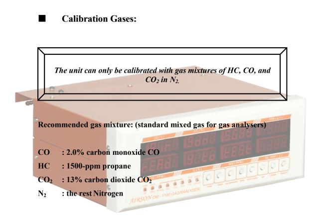
CO<sub>2</sub> should be present in the calibration gas to minimize the CO/CO<sub>2</sub> Quench effect by molecular collision processes.
